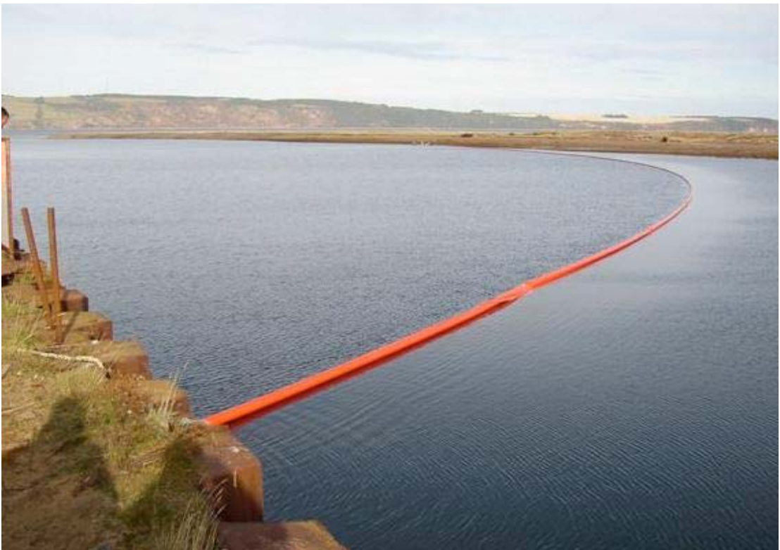
Figure 5 Deployment of a skirt boom
