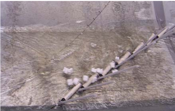
#6: Doesn't work-cantilever/ water over top
