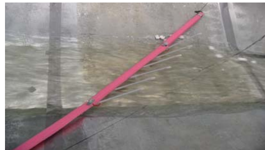
#10 (front): Floats/ velocity: low-works high-doesn't work
