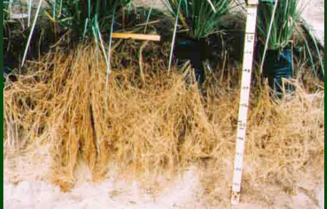
Malaysia - longitudinal section through hedge note the root mass in the top meter of the soil profile. This type of root mass will improve soil shear strength by up to 39%
